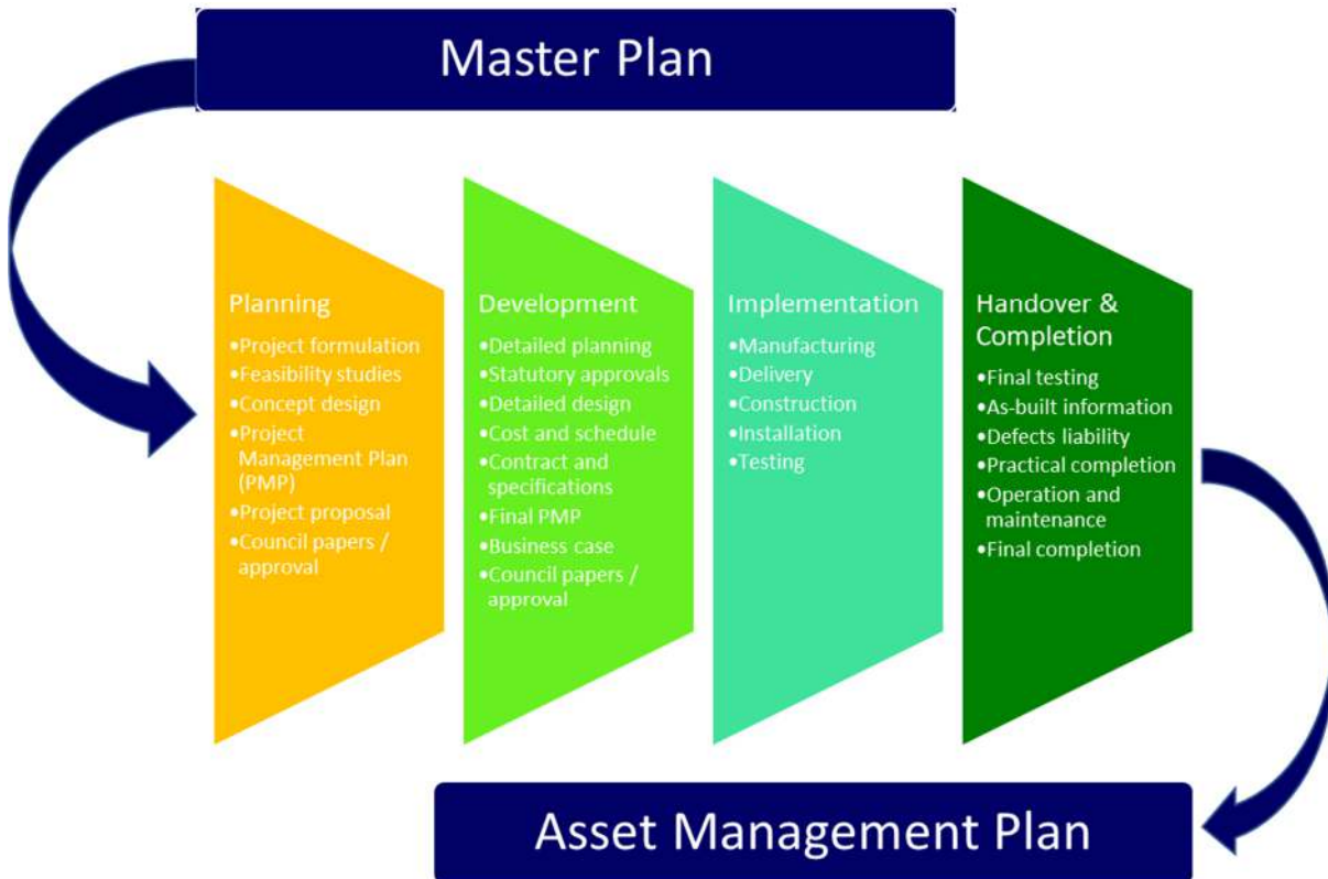
Figure 6.1 Airport infrastructure development flowchart
